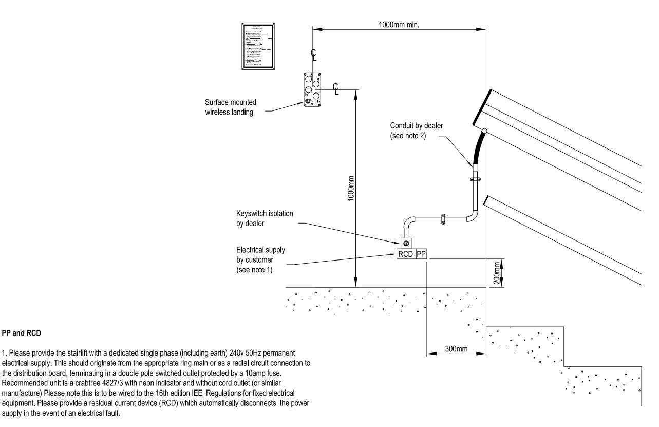
2. The conduit fitted by the installer is 20.0mm diameter plastic, which is surface mounted. If the customer requires the conduit to be in the wall prior to installing the lift. Then customer must provide two draw strings in the conduit to allow for the installer to pull the cables through.
